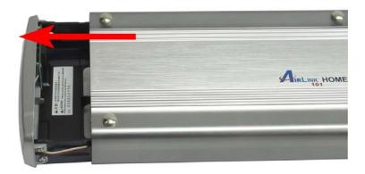
**Step 3** Put the 3.5-inch IDE hard disk into the plate, and connect the IDE and power cables to your hard drive.
